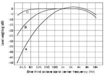
Figure 1.9. Frequency weighting characteristics for A and C networks
