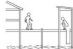
Overhung latrine — severe health risks, particularly for downstream users.
