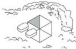
Shallow pit — flies and hookworm problems.
