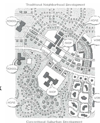
Figure 15.4 Schematic Comparison of Street Networks and Land Use in a Traditional Neighborhood and in an Area of Sprawl
